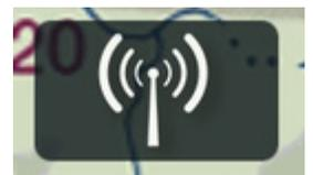
Tapping on the ADS-B receiver icon will reveal various status information for your receiver including firmware version and GPS received data.
